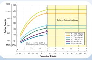
Cooling capacity based on chillers with P2 pumps set at 10 gpm. Other pumps and flow rates will affect cooling capacity performance.
