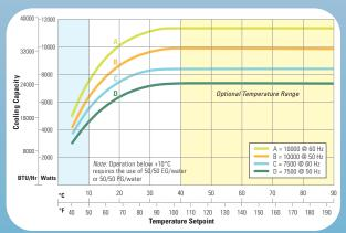
Cooling capacity based on chillers with P2 pumps with no backpressure. Other pumps will affect cooling capacity performance
