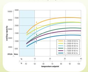
Cooling capacity based on chiller with P3 pumps with no backpressure. Other pumps will affect cooling capacity performance.
